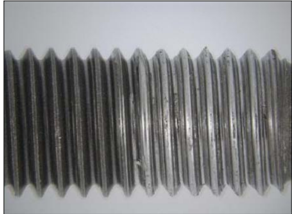
Photo 9. New exemplar stud – Left side original threads, right side after 10 installation/removal cycles using the same nut.
