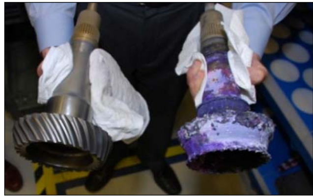
Photo 6. Damaged tail take-off pinion on right
